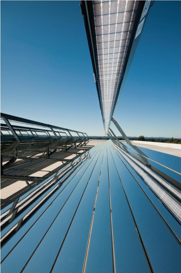
Figure 1: A single Cogenra SunDeck® module, which includes a collector area comprised of staggered flat mirror segments arranged in a parabolic arc and a PV/thermal receiver.
