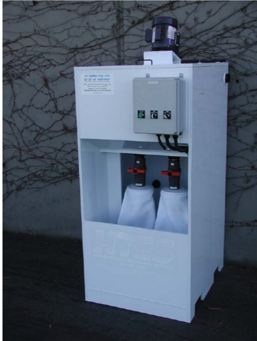
50 Gallon Semi-Auto Batch system with bag filters
